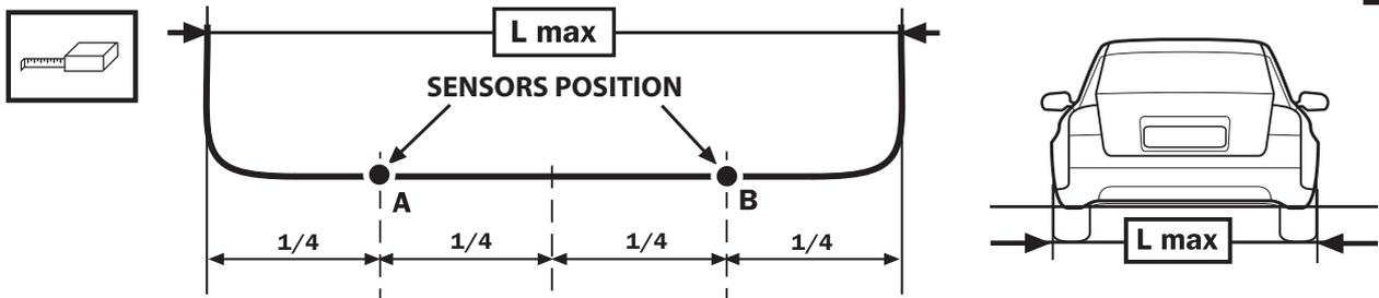
To achieve the best performance it is advisable to put the sensors in symmetry between each-other as shown in fig.4, the distance between sensors can vary from a minimum of 30 cm to a maximum of 60 cm. In case it would not be possible, it is very important to evaluate the position of the capsules and consider their range of action to consequently adjust the sensitivity of the parking system.
